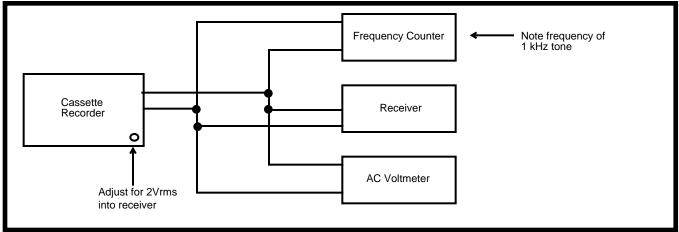
Figure 1 - Test Setup - Calibration Test
