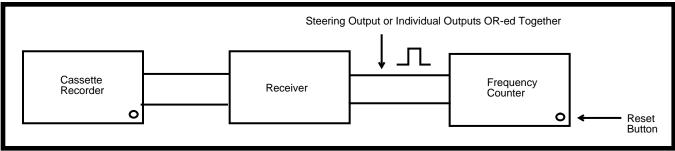
Figure 2 - Test Setup - Receiver Test
